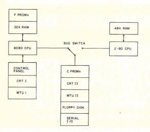
Fig. 1. A simplified block diagram of the computer system used to illustrate the functioning of the Memory Map program. Two processors share a block of memory and I/O resources. happened I thought it was rather funny.
